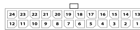
Fuel Controller Connector as seen on the unit itself Consult PIN OUT table for more information
